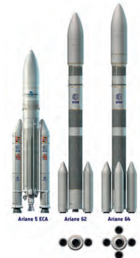
Ariane 5 vs Ariane 6.2 and 6.4 configurations
